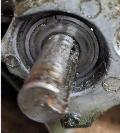
Internal tabbed washer. Remove it.
